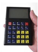
**Palmtec DataCol** is a hand-held computer It is very rugged, light weight with about 250 - 400 Grams and suitable for the rough environments. It consists of Key keypad, Graphic LCD, Basic & In Built **Scanner / BIOMETRIC MODULE** etc, Higher End 32 Bit Microcontroller, USB and runs on Battery.
